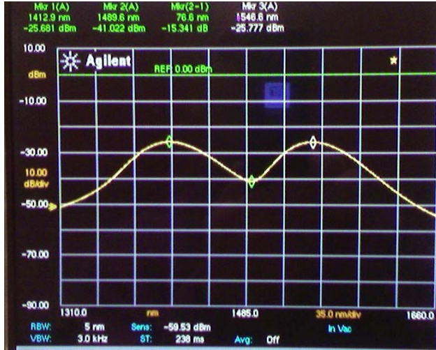
Fig. 1: Source spectrum, 1310-1660 nm
